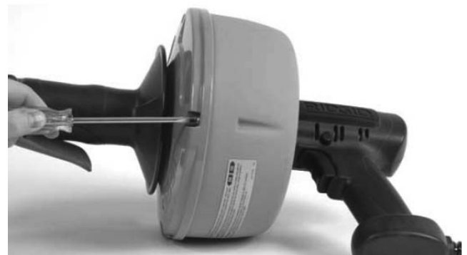
Figure 6 – Loosen Four (4) Screws From Back Half of Canister About Three (3) Full Turns
